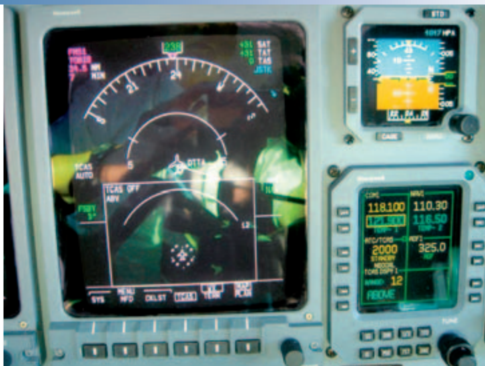
→ TCAS display showing TCAS off and transponder on stand-by on the RMU.
